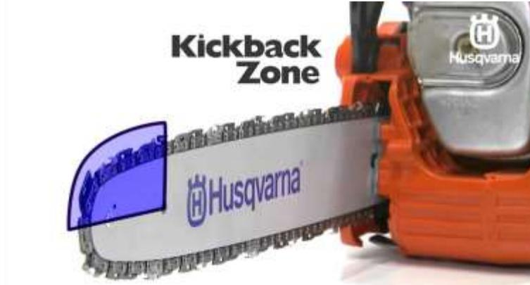
6. Always stand so that you are looking at the left side of the bar. If you can see the right hand side of the bar it means you are bent over the saw and what then if the saw does happen to kick? Your neck is exposed. You need your neck to keep your head in place so protect it!
