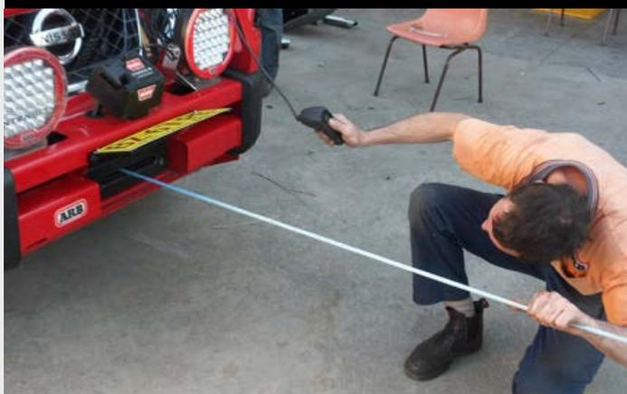
Don't ever let out all your rope when winching. Leave at least one layer on the drum or else your winch won't work at maximum efficiency. Grab an extension strap instead of going all the way to the bare drum.
