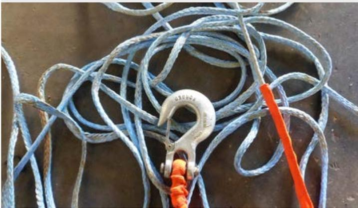
Let the rope dry for a bit before winding it back on, but don't leave it in the bright sun for too long. Ultra-violet light will degrade synthetic rope.
