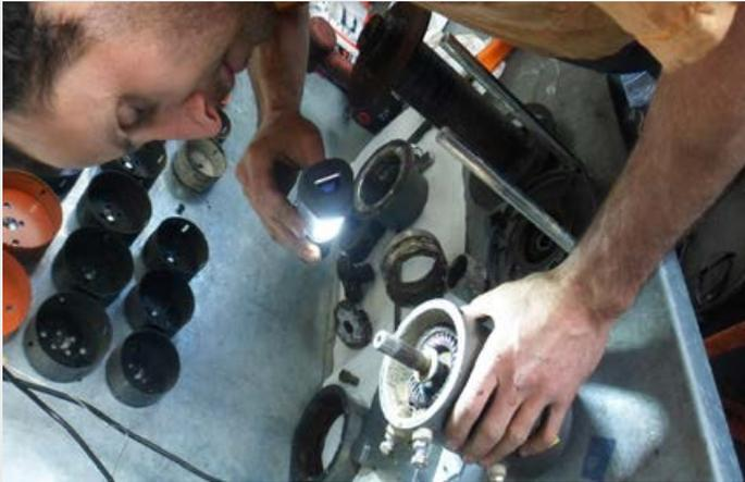
Get your winch serviced every two years. ARB does a winch service for about \$300. If you are doing it yourself, thoroughly clean everything, remove any corrosion and give it a coating of high-temperature grease.
