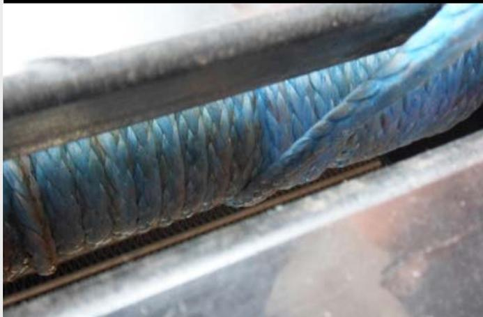
Make sure the rope is wound evenly and neatly back onto the drum. Unevenly spooled rope (where it creates a "bird's nest" at one end of the drum) can similarly reduce the pulling power of your winch and lead to overheating problems.
